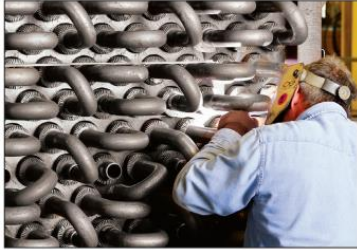
STANDARD DESIGN INCLUDES AN INTEGRAL ECONOMIZER FOR ENHANCED HEAT RECOVERY.
